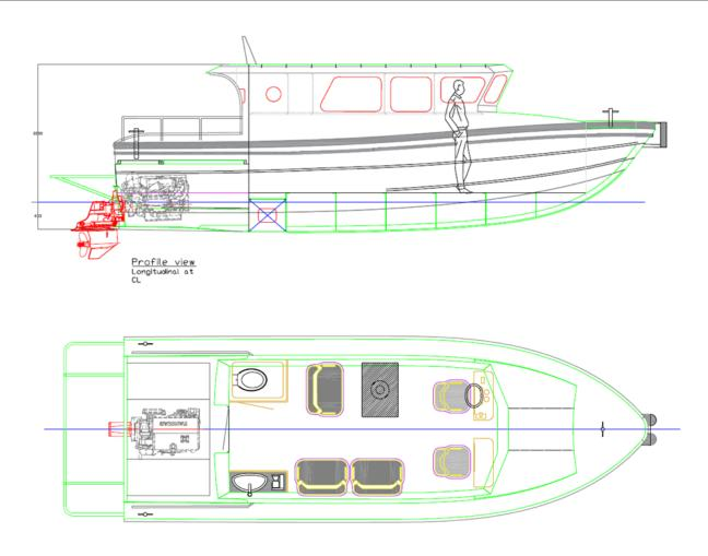
Drawings above are based on a 10 meter version. The 12 meter version will have a extended hull and large cabin where in the front section we will create space for 3 beds. Plus engine room will base twin inboard diesel with V-drive.
