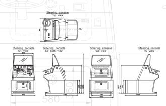
All GRP consoles are standard made by the hand lay-up process. On request with vacuum injection and divinycell core. Colour on request.
