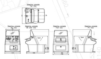
All GRP consoles are standard made by the hand lay-up process. On request with vacuum injection and divinycell core. Colour on request.
