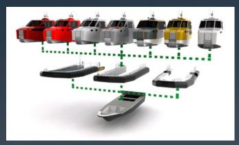
The client can choose between several cabins and fender types, this makes the boat suitable for almost any purpose. The cabin can vary in length and the interior and deck layout are fully custom.
