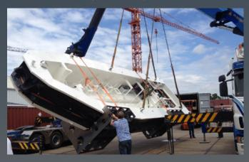
The MPRV can be used for projects worldwide due to the re-attachable cabin. The hull and cabin are shipped around the world in 2 standard open top containers.
